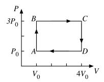
3. A sample containing three moles of an ideal gas is taken through a series of equilibrium states, as represented by the closed path ABCDA in the diagram above.
