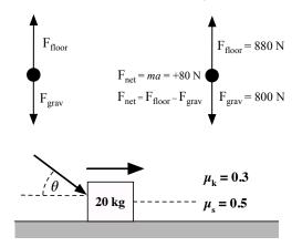
12. This crate is being pushed along a floor by a handle that exerts 50 N on the box at an angle of 37° as shown above. The coefficients of friction between the crate and the floor are  $\mu_k = 0.3$  and  $\mu_s = 0.5$ . First sketch the force diagram. Use it to guide us in filling out the "force table" to the right:
