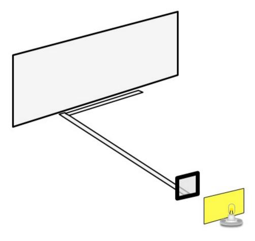
A lamp with a tiny filament shines through a yellow filter and then through a diffraction grating with its lines ruled in the vertical direction. The grating is held at one end of a meter stick which is aligned with the lamp. At the other end of the meter stick, a second rule is placed at right angles to the first rule.
