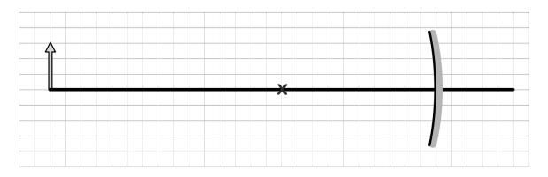
14. An object is placed 50 cm from a concave mirror that has a focal length of 20 cm as shown above.
