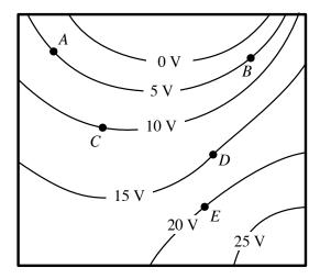
The diagram above shows equipotential lines in a plane produced by a distribution of electric charge. Points A, B, C, D, and E are all in the same plane as these equipotentials.
