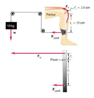
10. A device for exercising the upper leg muscle is shown above along with its free-body diagram. Calculate the force exerted by the upper leg muscle to lift the 10 kg mass at a constant speed.
