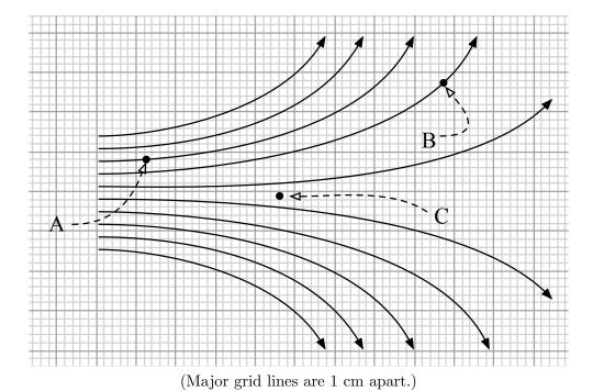
An electric field is established in a vacuum as represented by the field line diagram above.
